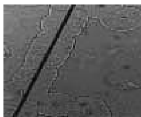
Fig. 2. Transcrystalline morphology in CT/mPP model composites ( t=8\text{min} , T_c=124\text{ }^\circ\text{C} , \times 200 )
